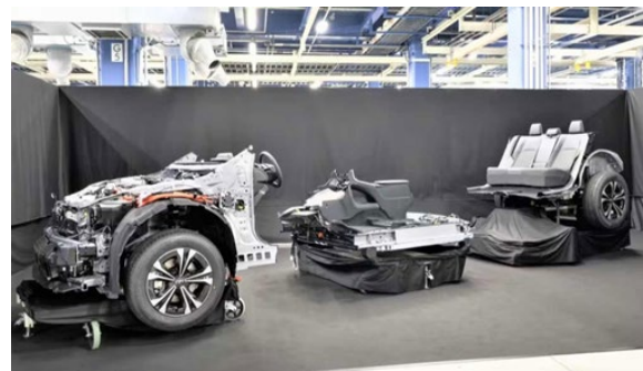
Figure 14. Gigacasting will be used to make the front and rear sections of the new electric model due out in 2026. 7
