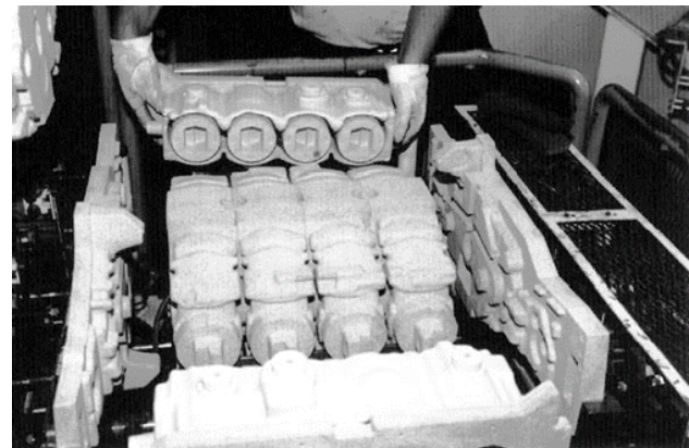
Figure 6. Core package with gluing fixture drawbacks in place against the outside of the assembly. Note the shell breather core on top of the package.
